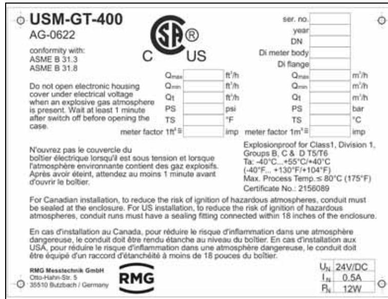
Fig. 13-3: Type plate NEC (CSA)
