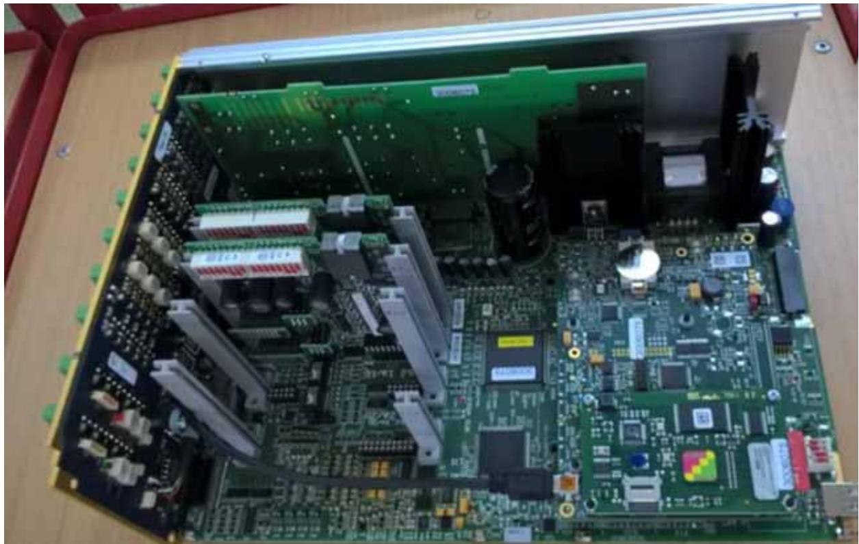
Fig. 8-21: Slot for the option card with COM 6 and 7 of the ERZ 2000-NG
