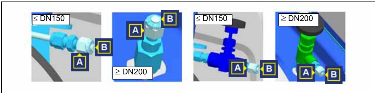
A Union nut with clamping screw connection (A)
