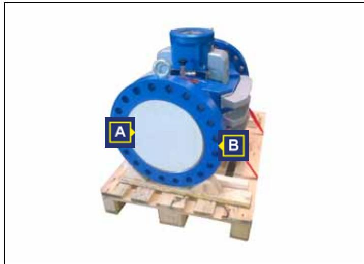
*Fig. 6-5: Removing the protective sticker*
