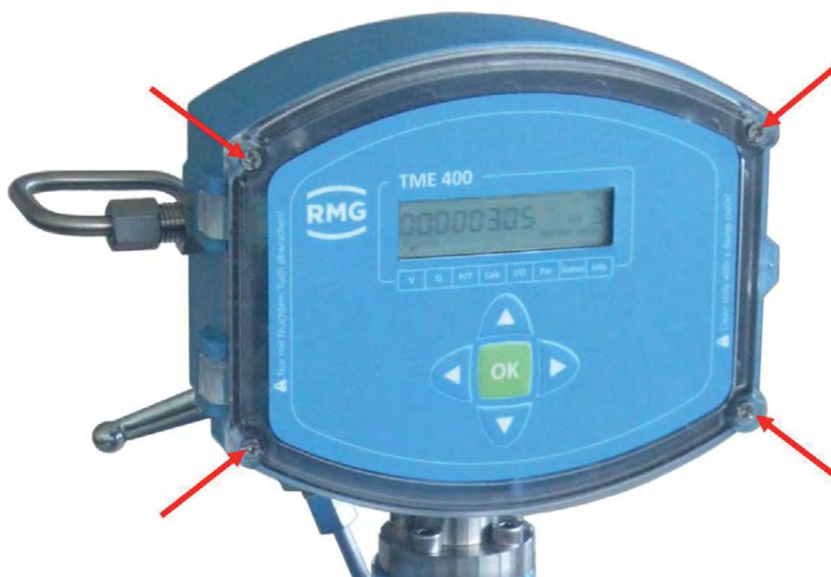
Figure 3: Unscrewing the screws to open the cover
