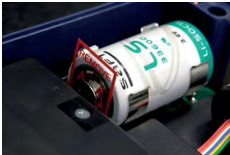
Fig. 15: Removable foil strip at battery holder
