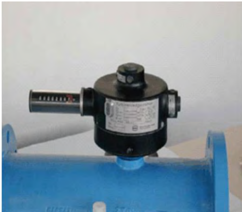
Figure 6: Type “D” meter head
