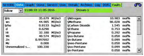
This screen displays the results of the last analysis, the molar content of the gas components in the right window and values such as calorific value, standard density and Wobbe index that calculated from the molar content in the left window. The methane number is also shown if its calculation is activated.
