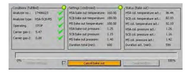
After termination of the heating process, cooling is started immediately. Now no more actions and interventions in the cooling process are possible and the cooling time (always 1 hour) has to be waited.
