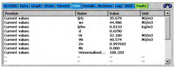
The user screen offers the possibility of summarizing 20 arbitrary, frequently needed measurements for quick display.
