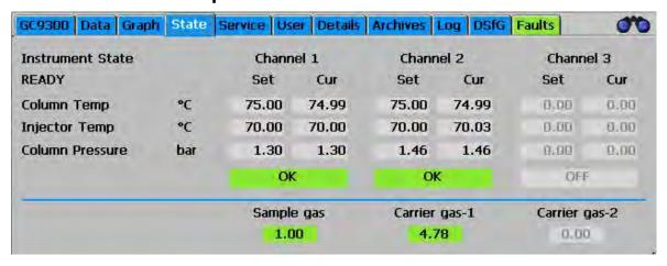
Variables such as pressure and temperature for Columns 1 to 3 and inlet pressures for measuring gas and carrier gas can be found here for the entries in the maintenance log. An additional, second carrier gas is used for some applications.
