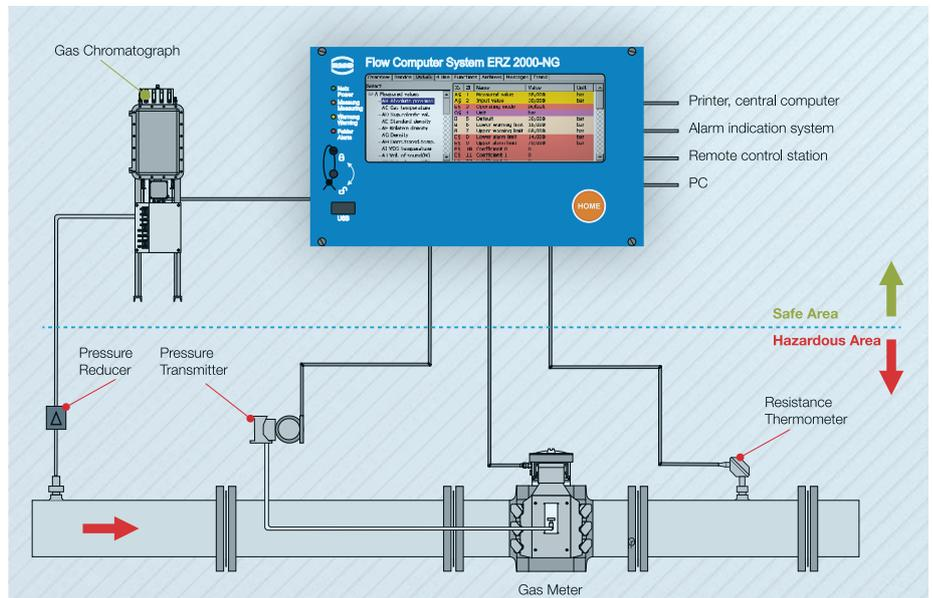
The ERZ 2000-NG base module performs neutral measurements of all inputs similar to a multimeter, but no calculations or assignments to physical units are made.
