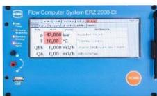
Experience makes RMG a leading supplier in natural gas measurement. This is also evident in the ERZ 2000-DI flow computer - a volume corrector that is specially tailored to the needs of distribution network operation.
