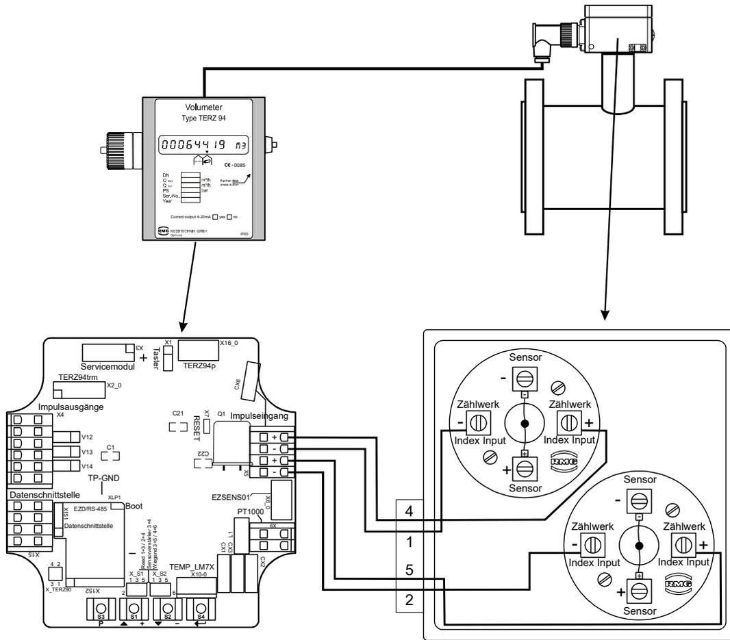
If your TERZ 94 is designed for remote totalizing, you can install the totalizing unit at a distance of up to 50 m from the meter case. Usually, the cable has already been connected to the totalizing unit when the TERZ 94 is delivered. Should this not be the case, you will have to connect the connecting cable to Input-terminal X5, clamp S1+ and clamp S1- of the board. For 2-channel meters connect the second sensor to the clamps S2+ and S2-. Use only shielded cables of the type:
