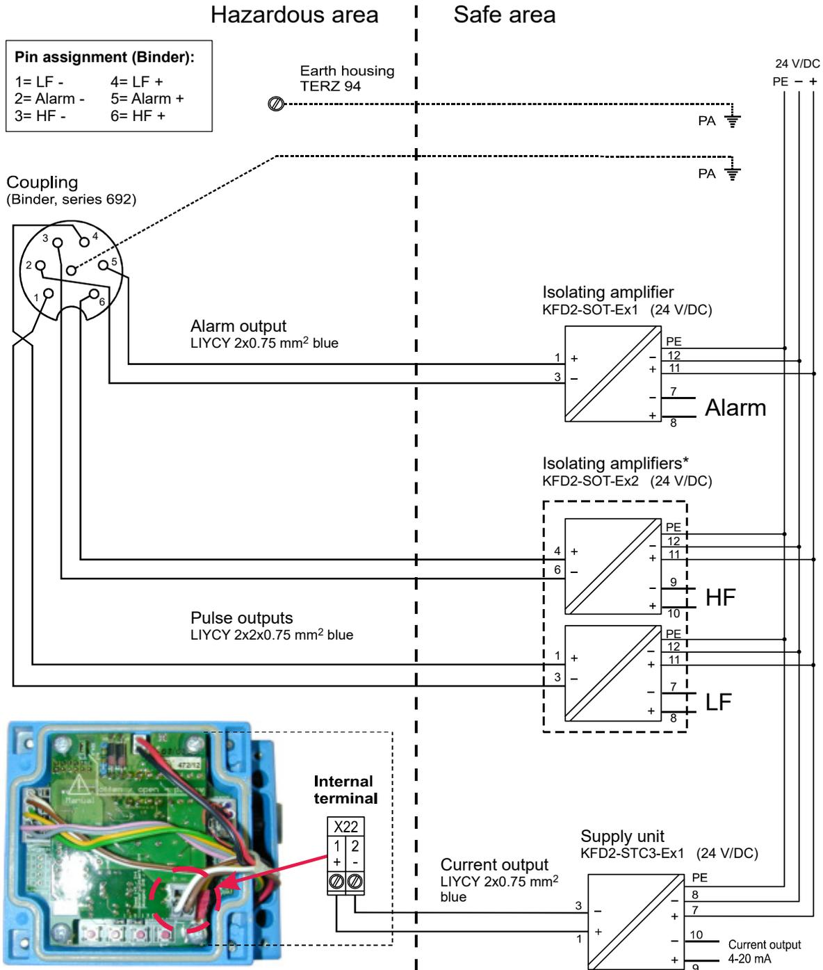
\* If 2-channel isolating amplifiers are used, the two inputs must be separated!
