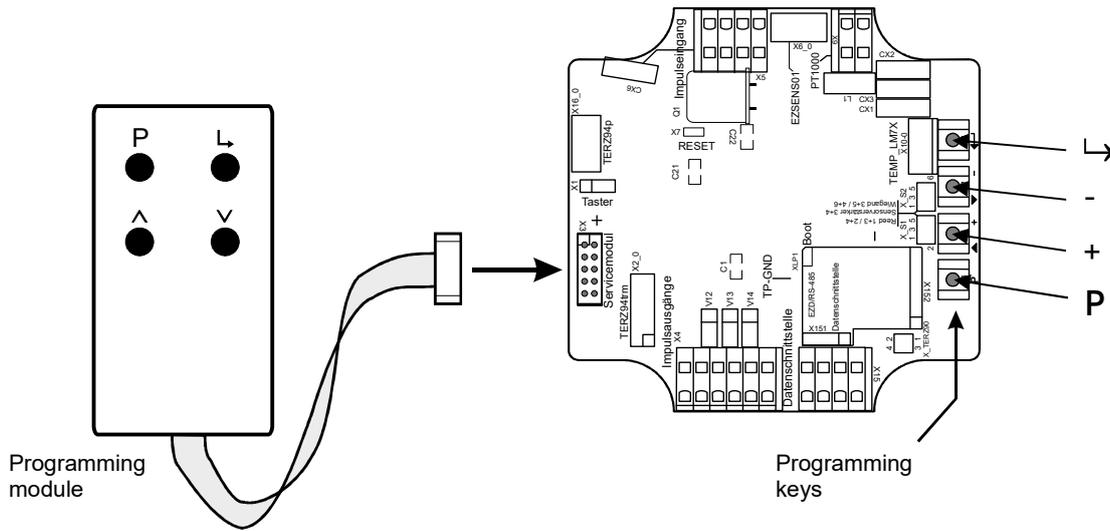
Programming with the programming module is to be performed in the same way as with the buttons.
