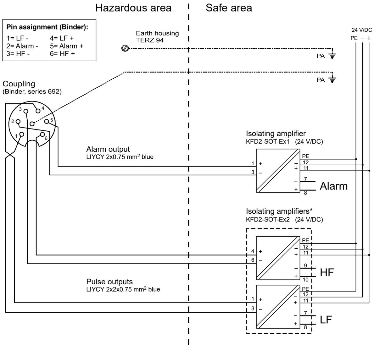
\* If 2-channel isolating amplifiers are used, the two inputs must be separated!
