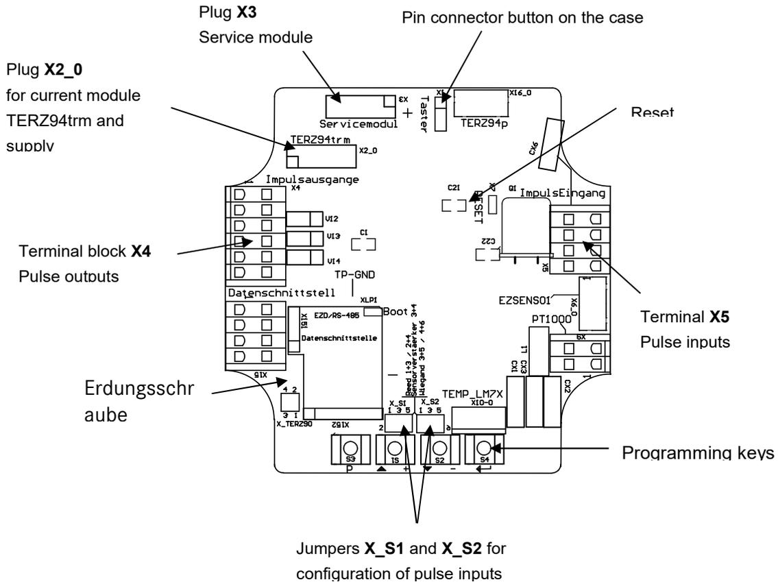
To convert from the meter head directly mounted on the meter case to the remote totalizing unit and vice versa it is necessary to change the positions of some jumpers (see inputs and outputs in the annex).
