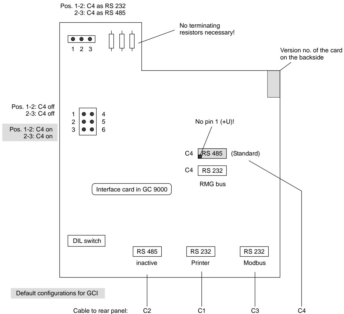
C4 needs external terminating resistors and a bus supply voltage (+5 V).
