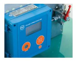
The EC 600 electronic volume corrector is a measuring instrument designed for the conversion of natural gas volume at measurement conditions to gas volume at base conditions. Information on gas volume passing through the device is measured using the impulse outputs of the gas meter. Integrated converters measure the gas temperature and pressure.
