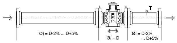
The inside diameters of the inlet and outlet pipes may be up to 2% smaller or up to 5% larger than the inside diameter of the meter.
