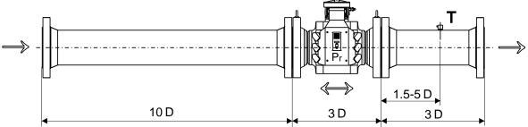
Standard installation without a flow straightener:
