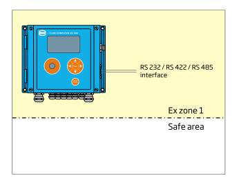
The EC 911 version is exclusively supplied by a lithium battery and has been approved for Ex zone 1 as an intrinsically safe device.
