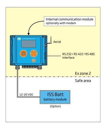
The EC 921 version is intended for use in Ex zone 2; it is not permissible to operate this device in Ex zone 1. It is supplied by two lithium batteries as standard: one for the corrector and the other for the internal communication module.
